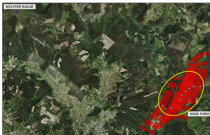
Fig. 8. Example of an aerial view showing the estimation of the scanning horizontal area where the wind farm may cause significant clutter level in a weather radar located at 7.7 km (represented as a blue dot) [61]. (For interpretation of the references to color in this figure legend, the reader is referred to the web version of this article.)
